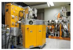
QAM, a compact sputtering system for thin-film deposition  $\ensuremath{\mathsf{R}\&\mathsf{D}}$
