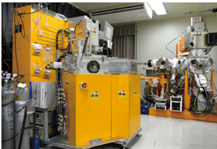
QAM, a compact sputtering system for thin-film deposition R&D
