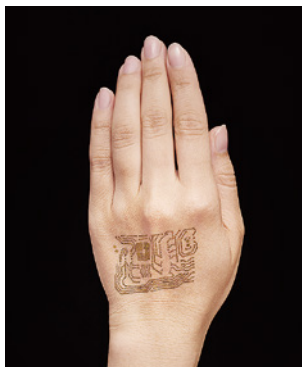
Figure 4: Wearable nanomesh electrode applied to the back of a hand. The electrode closely follows the skin contours. It lets the skin breathe naturally and is so thin and light that wearers forget they have it on.
