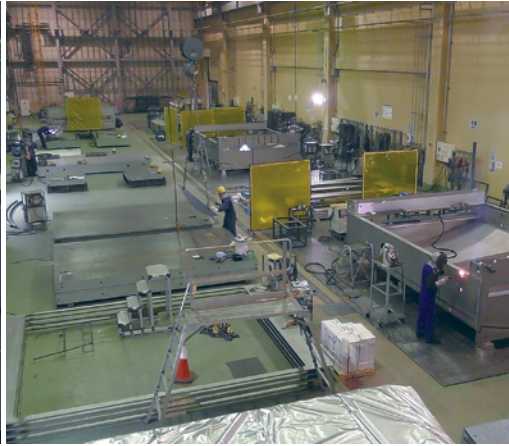
Soldering sites with multiple vacuum chambers
