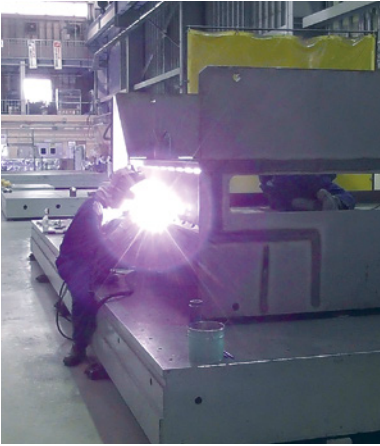
Vacuum chamber soldering
