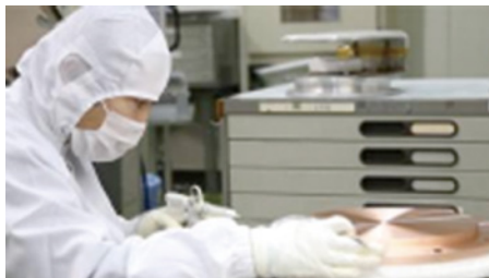
Testing sputtering target material
