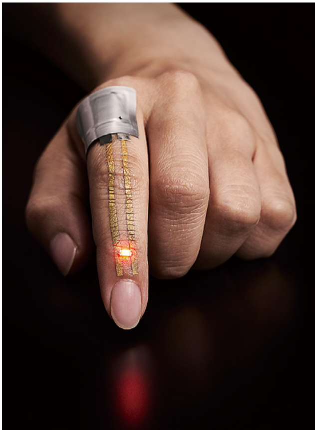
Figure 1: Wearable nanomesh electrode affixed to an index finger, with power supplied from a flexible battery that turns on an LED
