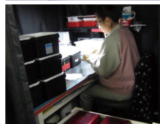
Mask blanks for semiconductors (top) Each glass substrate sheet is visually inspected in a dark room to check for scratches (bottom)
