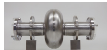
Single-cell accelerating cavity manufactured by KEK from ULVAC’s material
