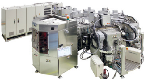
Sputtering system model SME-200
