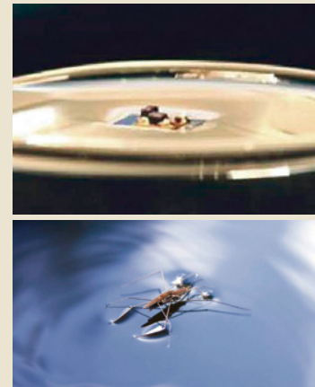
Photograph of a self-propelled microrobot powered by electricity that is transmitted by electromagnetic resonance (pond-skater robot) (above). Photograph of a pond-skater (below).
