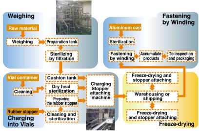
Flowchart of process for producing freeze-dried formulation
