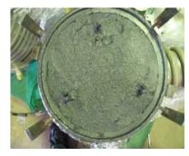
Here, apply a uniform coat of heat-transfer-cement about 1 cm inside the end.
