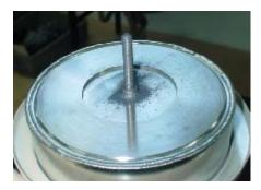
(2) Apply a uniform coat of heat-transfer-cement (item 7 of Table in 1.1.) to the bottom of the pump case.
