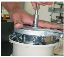
(5) Install the reflector (1) in position and tighten it with an M6 hexagonal nut (JIS Class 3).
