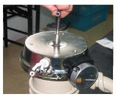
(8) Check and adjust the clearances between the heater terminal fixed position and the heater cover.
