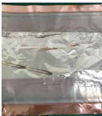
Fig.5 Picture of not treated Li surface that reacted with dry air.
