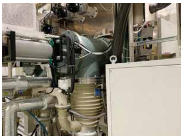
Fig.3 Roll to Roll Li evaporation system "EWK-030" and dry room.
