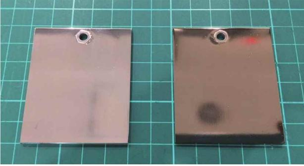
Figure 9 Nb substrates before and after coating.
