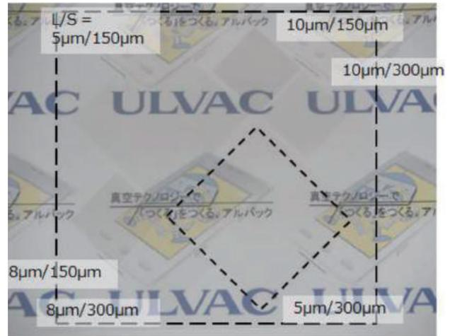
Figure 7 Image of the printed grid electrode.
