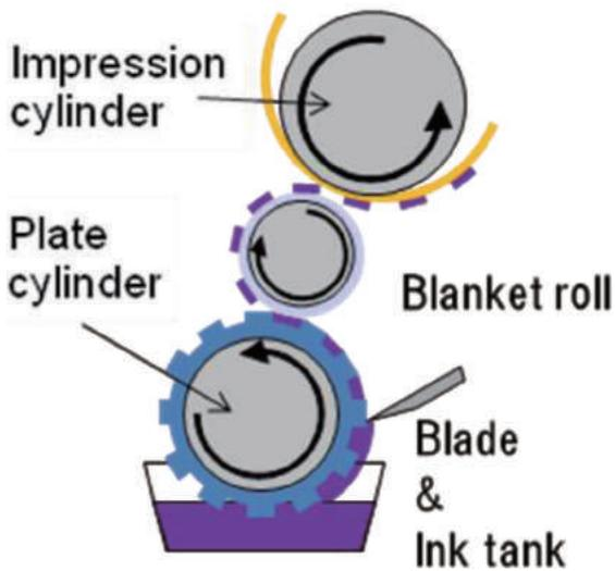
Figure 6 Schematic illustration of the gravure offset printing process.
