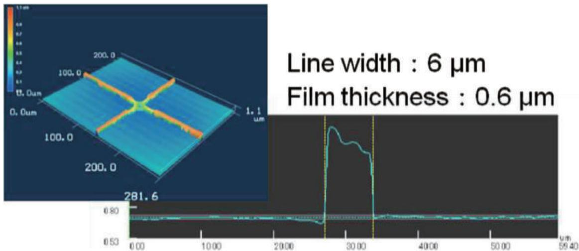
Figure 9 Wiring profile of the printed grid electrode.
