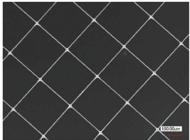
Figure 8 Optical microscope image of the printed grid electrode.
