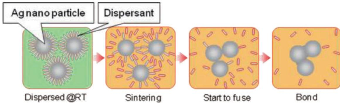
Figure 3 Sintering mechanism of the nano metal ink.
