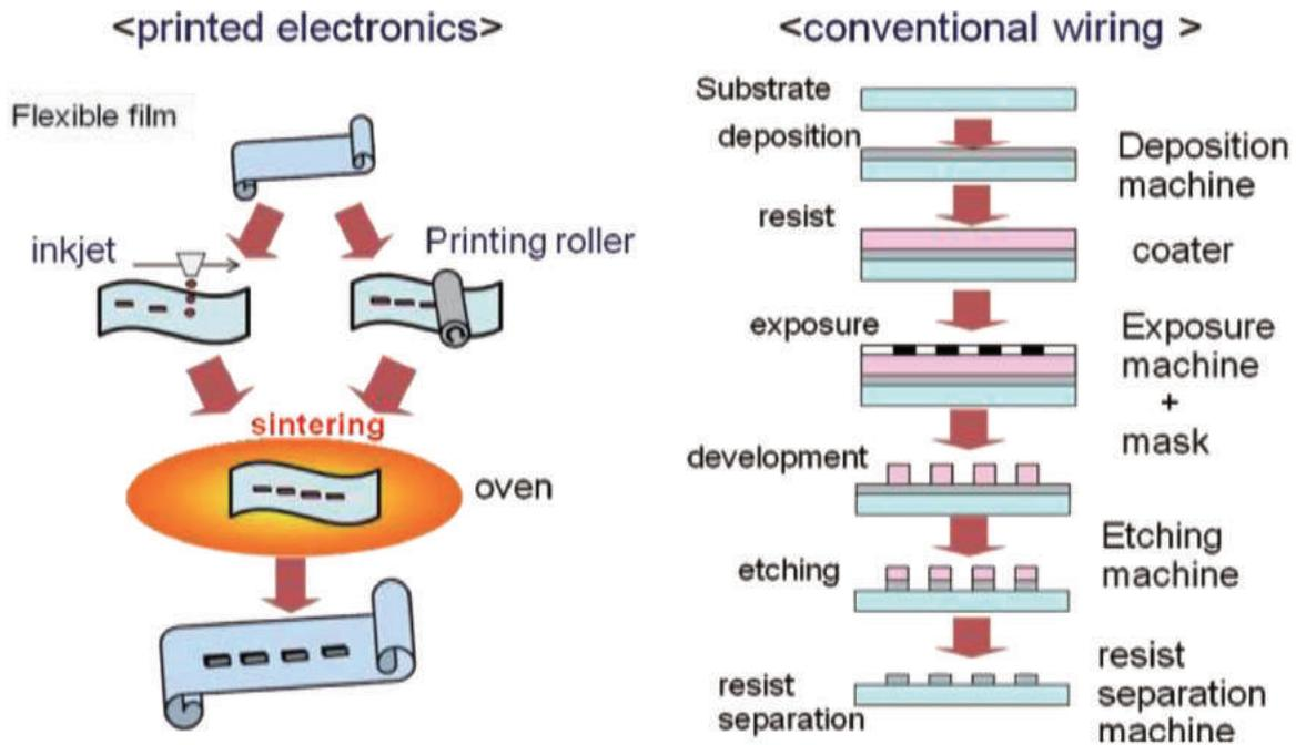
Figure 5 Comparison with conventional method and printing method.
