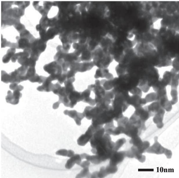
Figure 1 TEM image of typical Au nanoparticles.
