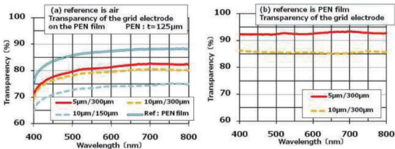
Figure 10 Optical transparencies of the printed grid electrodes on PEN film. (a) reference is air (b) reference is PEN film.
