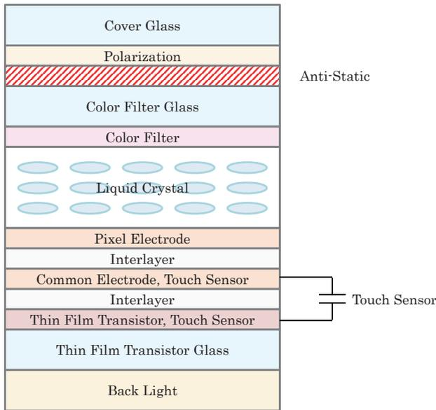
Figure 1 Structure of In-Cell type Touch Screen Panel.
