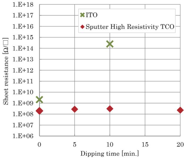
Figure 7 Chemical Corrosion Resistance Test.
