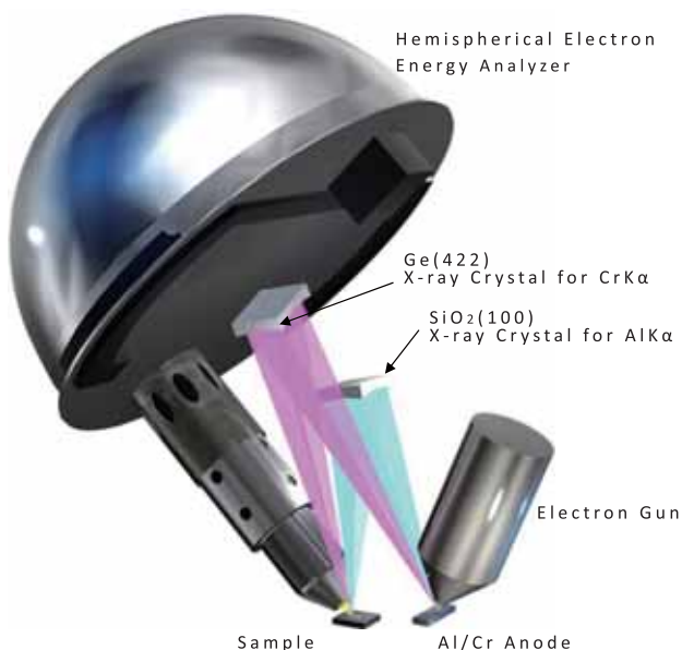
Figure 4 Schematic diagram of "PHI Quantes" optics.
