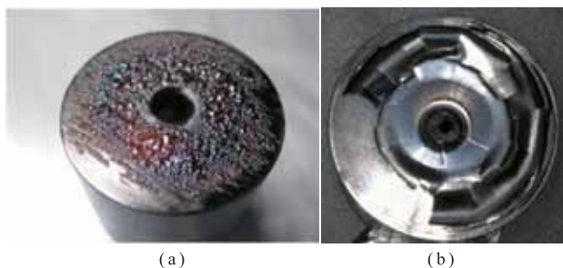
Figure 2 (a) Electrode of cold cathode ionization vacuum gauge when mounted and used directly above oil diffusion pump. (b) Electrode of cold cathode ionization vacuum gauge when argon gas was introduced up to about 1 Pa and operated continuously.
