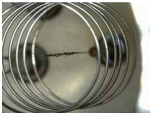
Figure 3 Ion collector of B-A ionization vacuum gauge whose indicated value is lowered.
