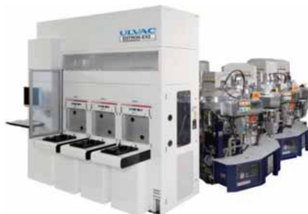
Figure 7 Reliable Emerging PVD Tool ENTRON EX W300 for STT-MRAM.
