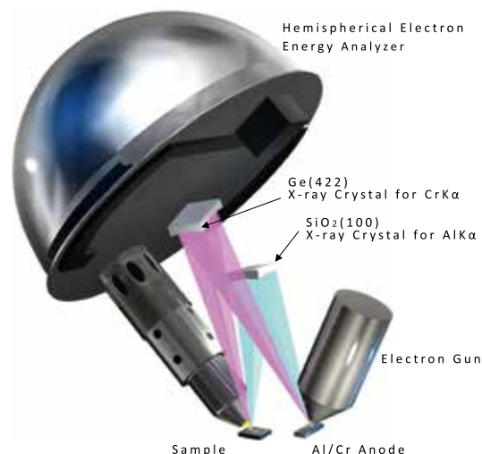
Figure 4 Schematic diagram of “PHI Quantes” optics.
