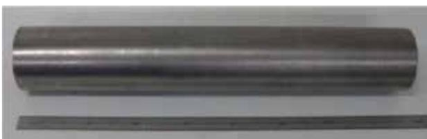
Figure 12 Niobium seamless tube for three cell cavity.
