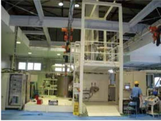
Figure 1 600 kW electron beam melting furnace.
