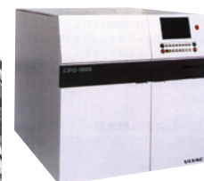
CPD-1000, a plasma CVD system that contributed to solar-cell development
