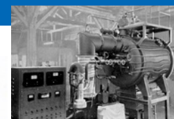
Uranium vacuum furnace, which was used later to produce high-performance materials, such as tantalum and titanium
