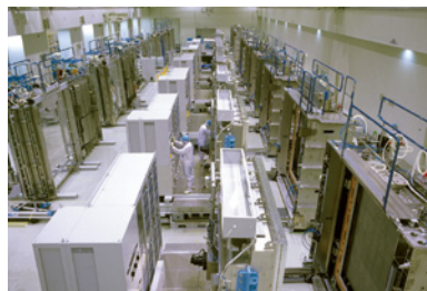
SMD-2400, the latest model of the sputtering system for TFT-LCD electrodes, which was awarded the 2006 ADY grand prix prize
