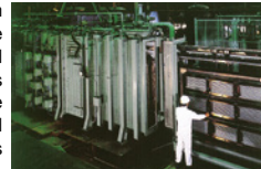
Aluminum vacuum brazing furnace that was developed for applications in the automobile and household appliance industries
