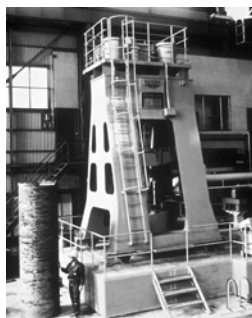
15-ton vacuum arc furnace, which delivers its full performance in various areas, such as the production of refractory active metals used for producing special alloys and in the space industry
