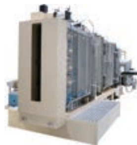
Cat-CVD equipment for silicon heterojunction solar cells
