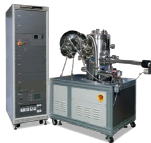
X-ray photoelectron spectroscopy equipment
