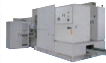
A capacitor is an electronic device that stores or discharges electricity to stabilize voltage and remove noise. One type of a capacitor is a "film capacitor" using very thin plastic film for automobile application. To deposit very thin layer of aluminum and zinc onto the thin plastic film (in vacuum) at tremendous high speed require state-of-the-art technology.
