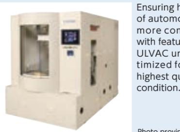
Ensuring high airtightness is important for the safety of automotive gasoline tanks. Plastic fuel tanks are more commonly used (compared to steel tanks) with features of lightness and design flexibility. ULVAC unique helium leak tester specifically optimized for plastic fuel tanks provide the world's highest quality measurement results in high vacuum condition.
