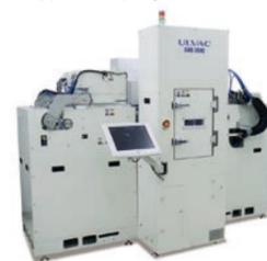
Sputtering equipment for electronic devices
