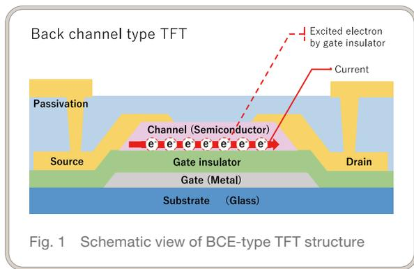
Fig. 1 Schematic view of BCE-type TFT structure
