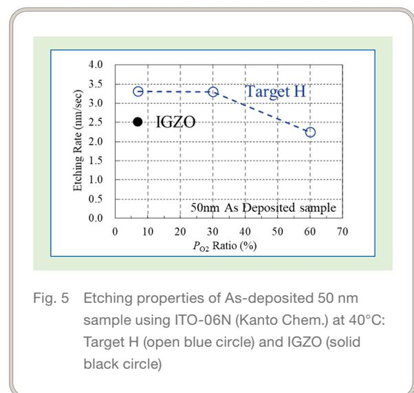
Fig. 5 Etching properties of As-deposited 50 nm sample using ITO-06N (Kanto Chem.) at 40°C: Target H (open blue circle) and IGZO (solid black circle)
