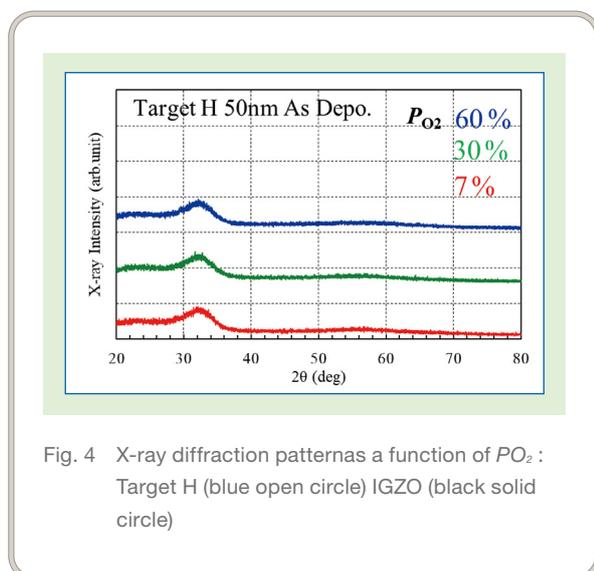
Fig. 4 X-ray diffraction patterns as a function of  $P_{O_2}$ : Target H (blue open circle) IGZO (black solid circle)
