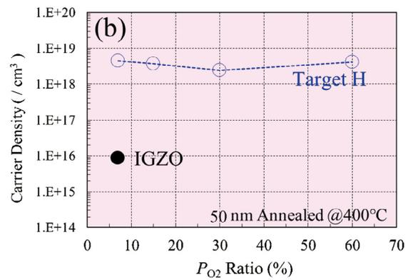
Fig. 6 Mobility (a) and carrier concentration (b) as a function of  $PO_2$ , estimated by Hall measurement: Target H (open blue circle) and IGZO (solid black circle)
