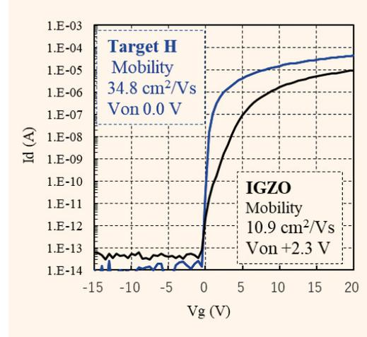
Fig. 8 I-V characteristics of BCE-type TFT: IGZO (black line) and Target H (blue line)
