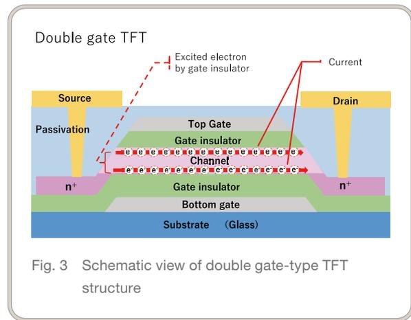
Fig. 3 Schematic view of double gate-type TFT structure
