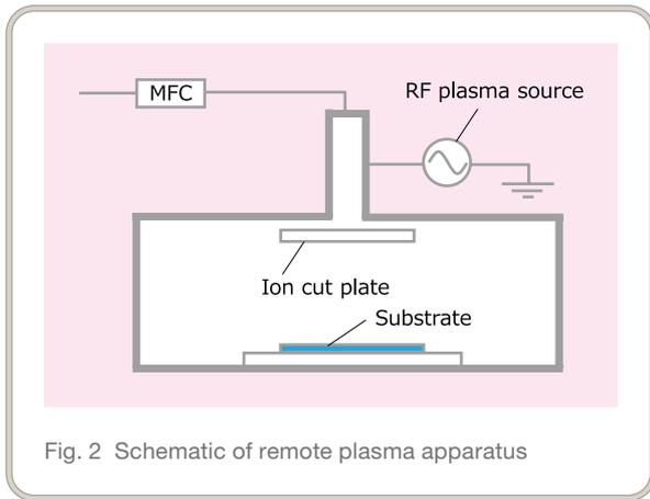
Fig. 2 Schematic of remote plasma apparatus
