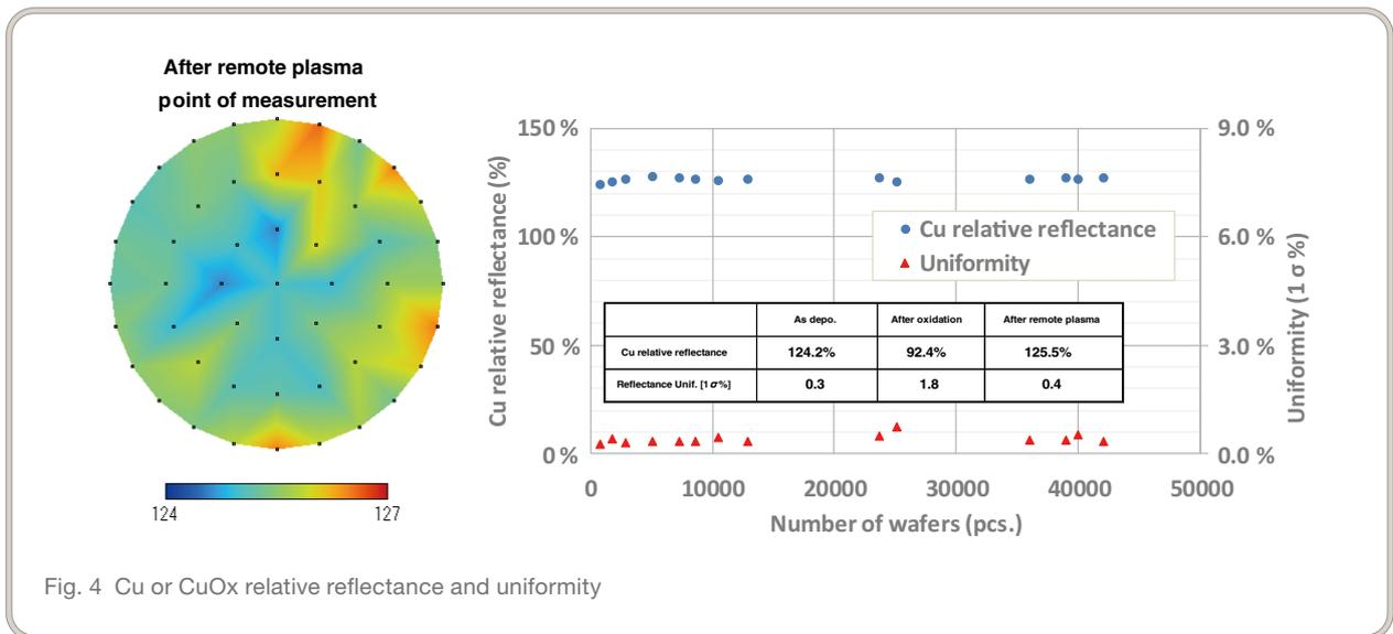
Fig. 4 Cu or CuOx relative reflectance and uniformity
