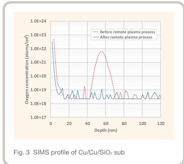
Fig. 3 SIMS profile of Cu/Cu/SiO<sub>2</sub> sub
