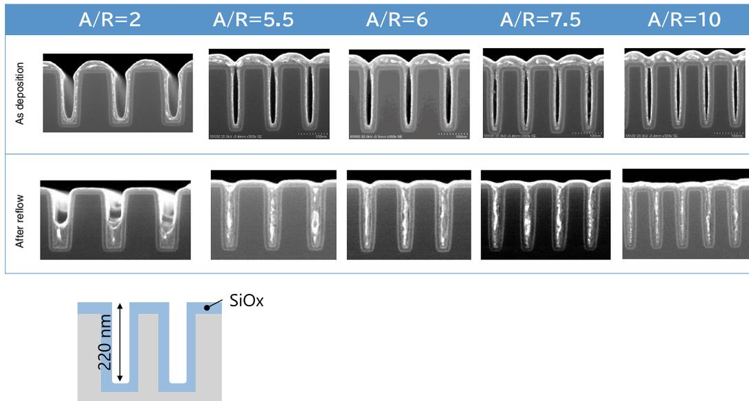
Fig. 12 Cu reflow margin
