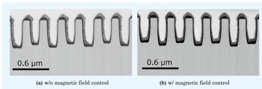
Fig. 6 Comparison of coating characteristics of Cu film with and without controlling the spatial magnetic field
