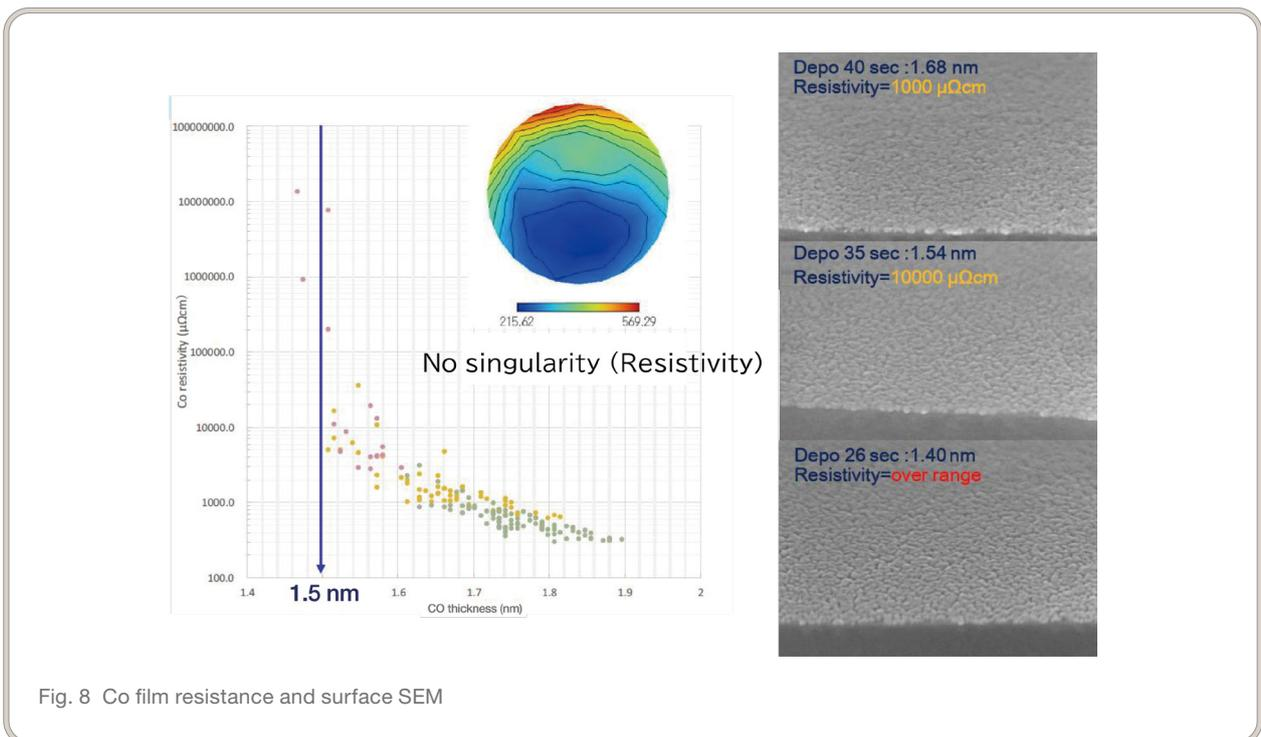
Fig. 8 Co film resistance and surface SEM
