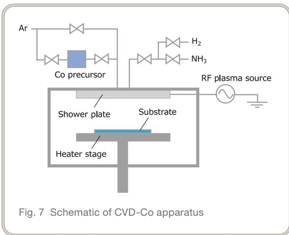
Fig. 7 Schematic of CVD-Co apparatus
