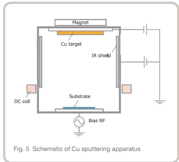
Fig. 5 Schematic of Cu sputtering apparatus
