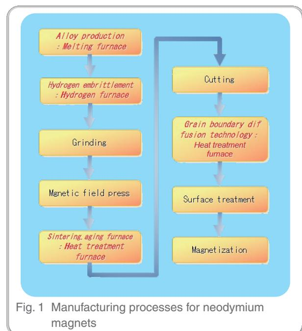
Fig. 1 Manufacturing processes for neodymium magnets
