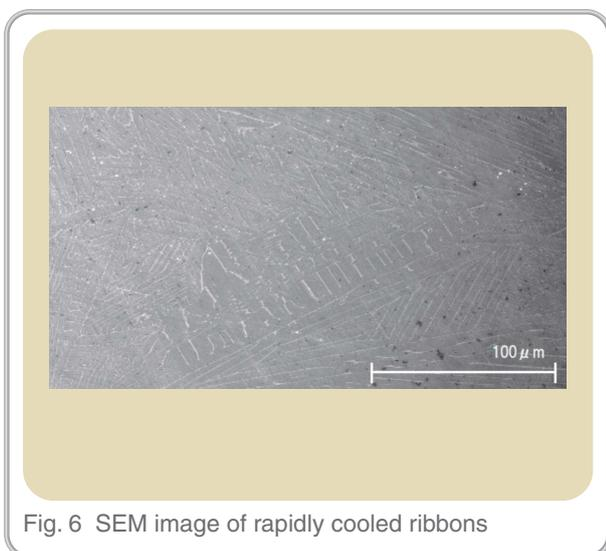
Fig. 6 SEM image of rapidly cooled ribbons
