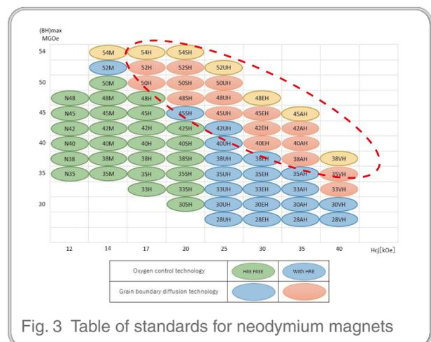
Fig. 3 Table of standards for neodymium magnets
