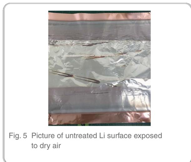
Fig. 5 Picture of untreated Li surface exposed to dry air
