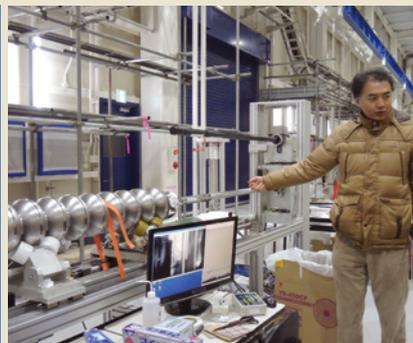
Superconducting accelerator cavity unit
