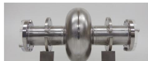
High-purity niobium materials for superconducting accelerators
