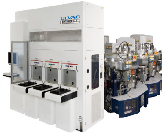
ENTRON™ EX2 W300 sputtering system
