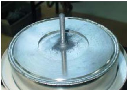
(2) Apply a uniform coat of heat-transfer-cement (item 7 of Table in 1.1.) to the bottom of the pump case.
