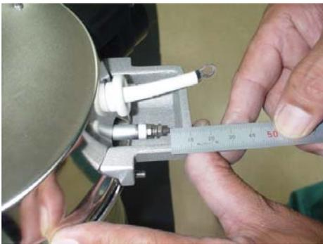
(9) Fix the heater lead using an M3 hexagonal nut, plain washer and spring washer. Retighten the M3 nut.
