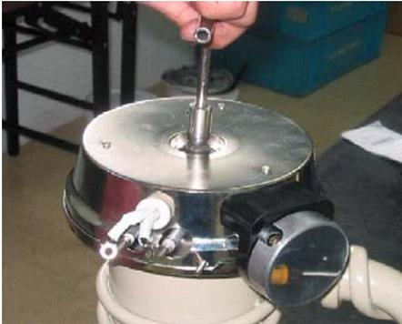
(8) Check and adjust the clearances between the heater terminal fixed position and the heater cover.
