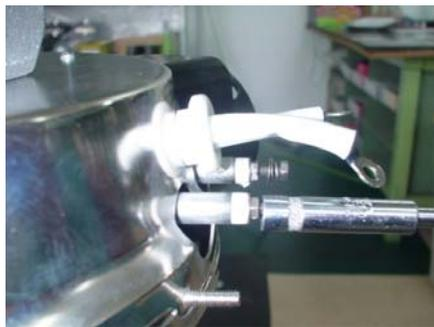
(10) Install the heater leads in parallel with each other, as shown in the photo.
