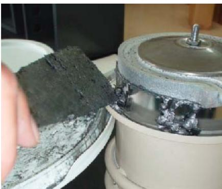
(7) Install the boiler cover in position. (M6 hexagonal nut and plain washer)
