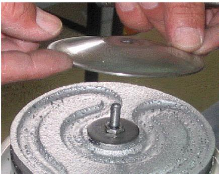
(6) Remove extra cement after allowing it to dry so that it does not stick to the pump case.
