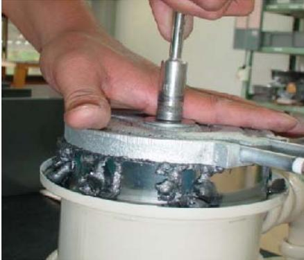
(5) Install the reflector (1) in position and tighten it with an M6 hexagonal nut (JIS Class 3).
