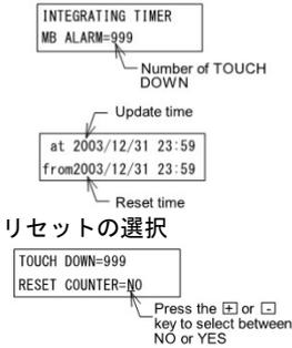
The number of warning that occur for the magnetic bearing system is counted.
