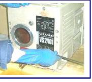
Step 4 Open the lubrication plug and fill fresh oil through it. (If a funnel is available at hand, oil can be filled without spilling it outside the pump.)
