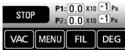
Figure19 Display of P1 and P2 output operation value on the Main screen
