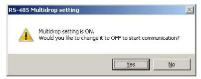
If "Yes" is selected here, change the multidrop setting to OFF and continue the connection processing. If "No" is selected, the connection process will be aborted.
