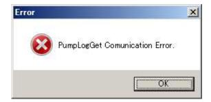
Check the connection cable to the pump and the serial port of the PC for any abnormality.
