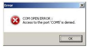
It is displayed when the specified communication port can not be used from this software. Make sure that the specified port is not used for other purposes.
