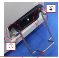
Power supply cord fixation metal appliance
