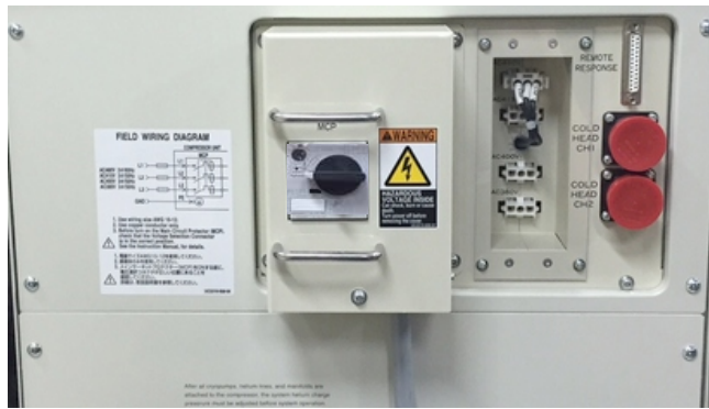
Figure 4-13 Close the Cover of Main Circuit Protector
