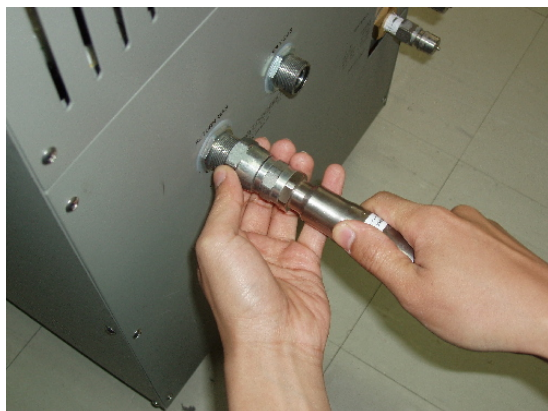
Figure 4-2 Tighten with Hands First
