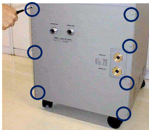
Figure 6-2 Remove All Seven Screws from the Rear Panel
