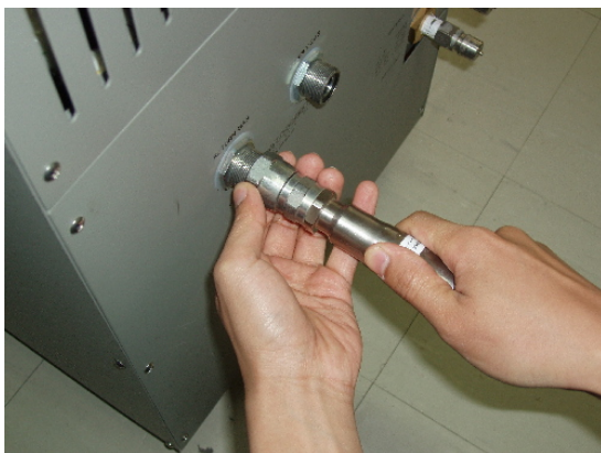
Figure 4-2 Tighten with Hands First
