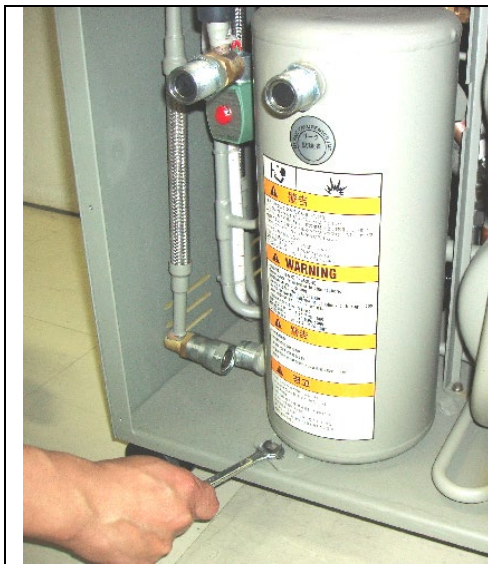
Figure 6-5 Connecting and Disconnecting Self-Sealing Coupling with Two Spanners
