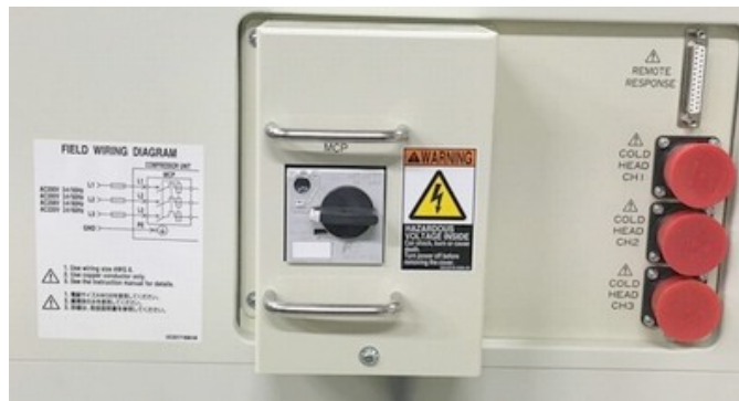
Figure 4-13 Close the Cover of Main Circuit Protector
