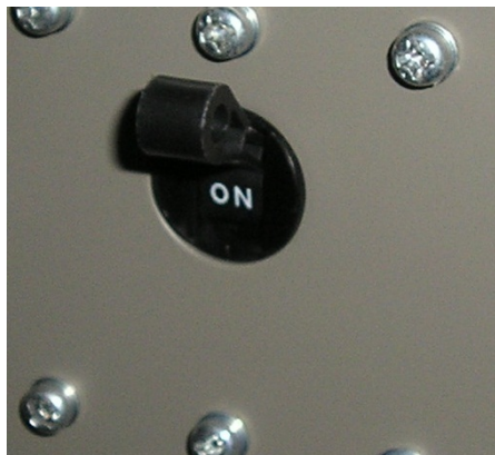
Figure A-3 P2 lever lifted up
