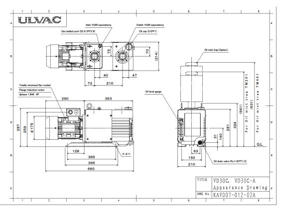
Fig. 4 Dimensional drawing VD30C, VD30C-F, VD30C-N
