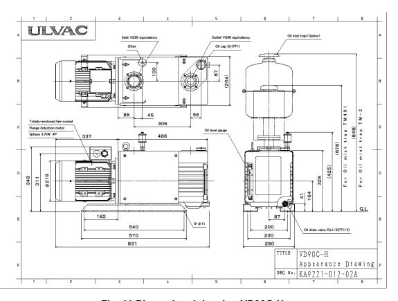
Fig. 11 Dimensional drawing VD90C-H
