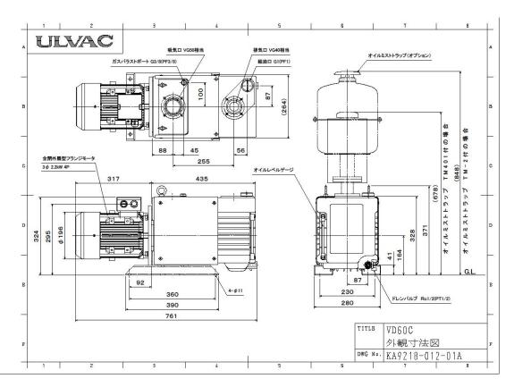
Fig. 6 Dimensional drawing VD60C
