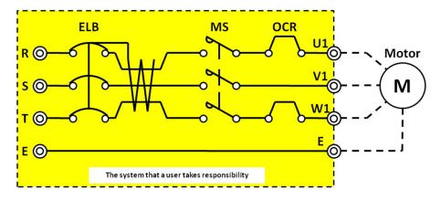
Fig. 16 Recommended connection diagram
