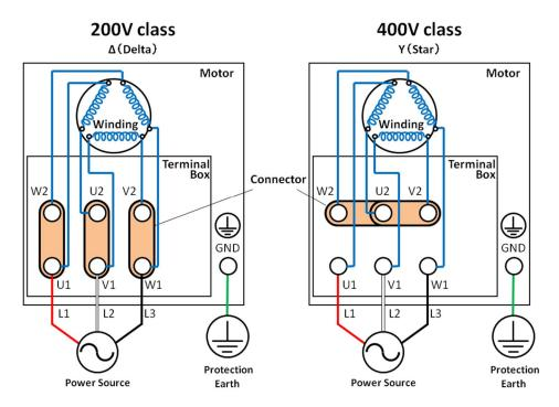
Fig. 17 Electrical wiring diagram
