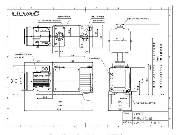
Fig. 7 Dimensional drawing VD90C
