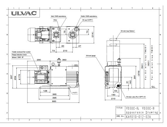
Fig. 8 Dimensional drawing VD30C-H, VD30C-B
