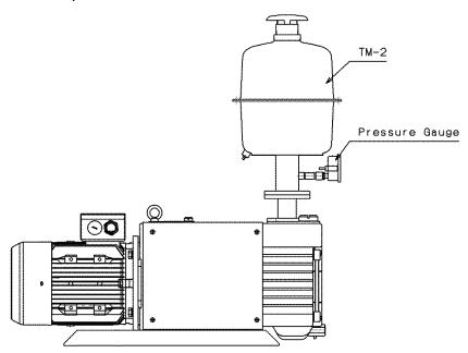
Fig. 18 Installation example VD90C
