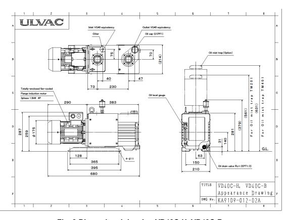
Fig. 9 Dimensional drawing VD40C-H, VD40C-B
