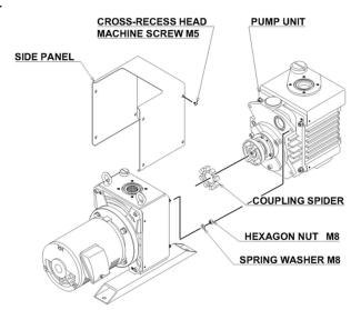
Fig. 19 Replacement of coupling spider
