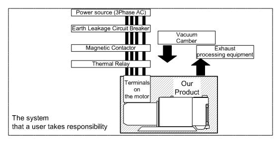
Fig. 3 Location of vacuum pump in host device
