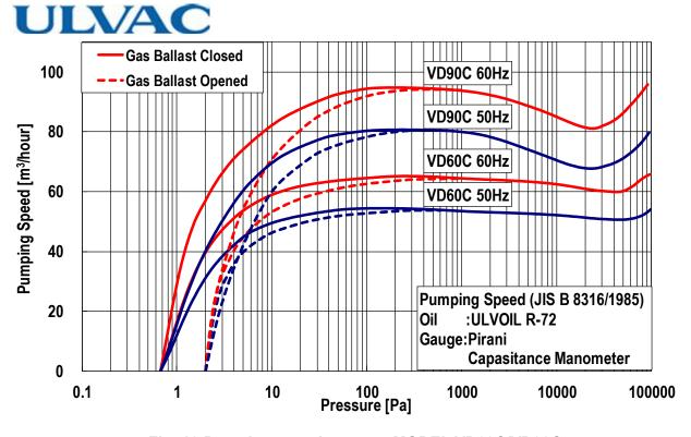
Fig. 13 Pumping speed curves - MODEL VD60C/VD90C
