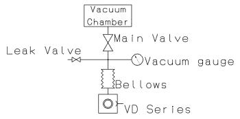
Fig. 15 Connection to vacuum chamber (example)
