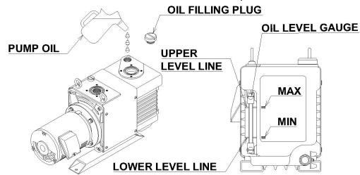
Fig. 14 Lubrication and oil level indication
