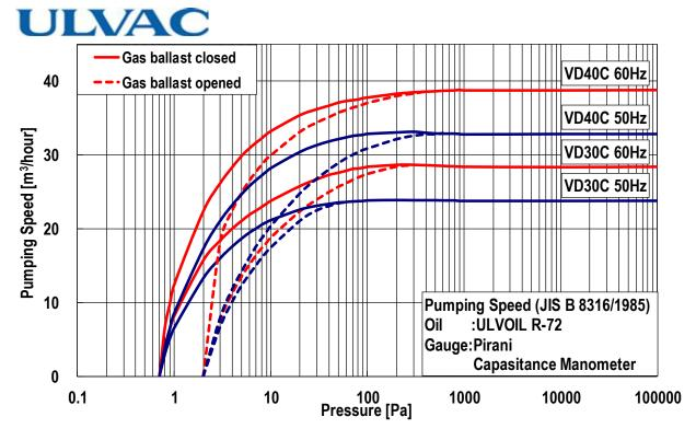
Fig. 12 Pumping speed curves - MODEL VD30C/VD40C
