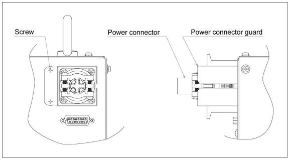
Fig. 23 Power connector guard attachment drawing
