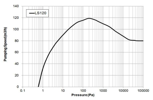
Fig. 5 Pumping speed curve (LS120)
