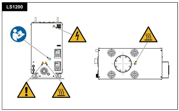
Fig. 4 Warning label attachment position (LS1200)
