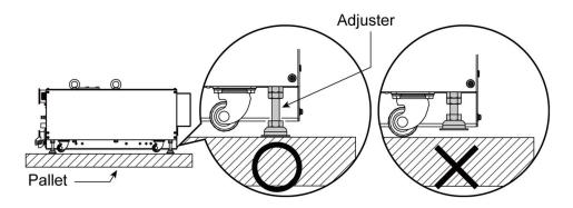
Fig. 18 Adjusters during transport
