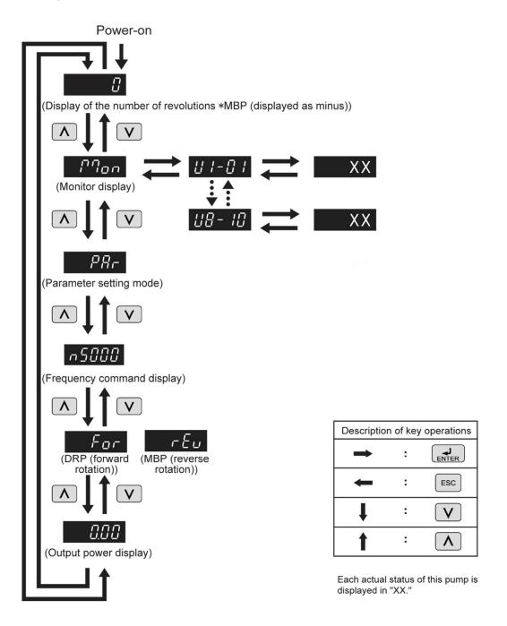
Fig. 14 Data display Transition diagram
