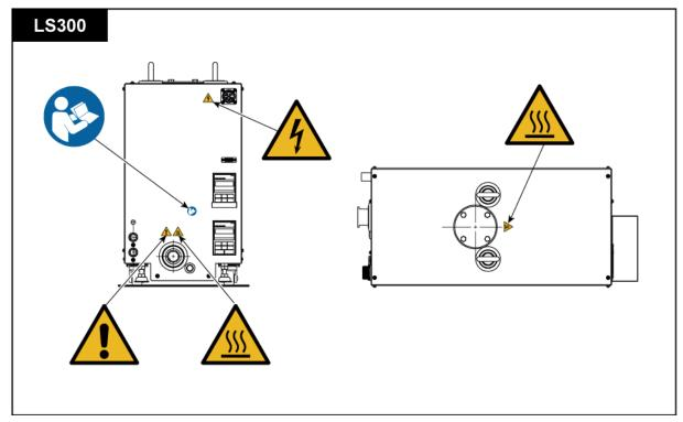
Fig. 2 Warning label attachment position (LS300)
