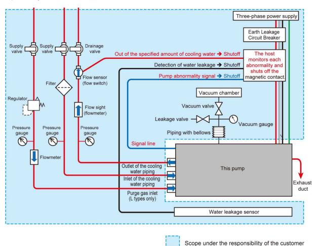
Fig. 15 System connection diagram
