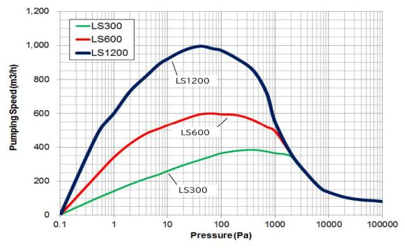
Fig. 6 Pumping speed curve (LS300, LS600, LS1200)
