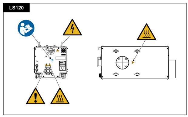
Fig. 1 Warning label attachment position (LS120)
