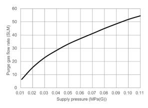
Fig. 20 Supply pressure and flow rate for regulator
