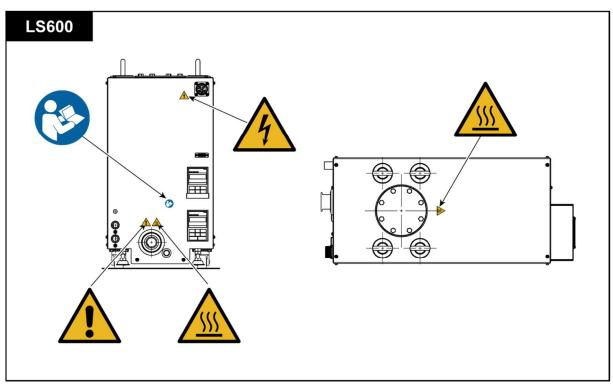
Fig. 3 Warning label attachment position (LS600)
