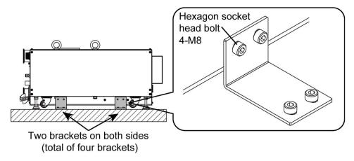
Fig. 19 Earthquake-resistant fixing brackets
