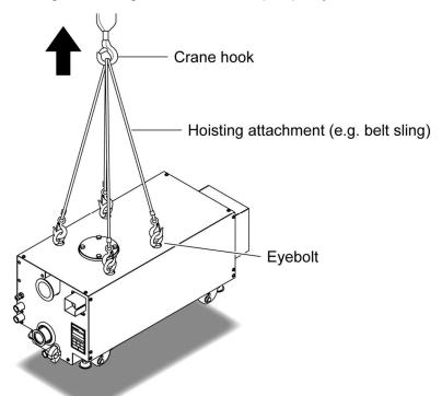
Fig. 16 Hoisting by crane
