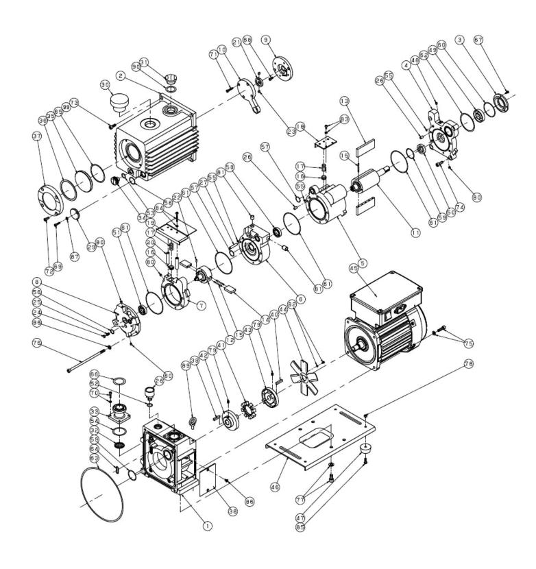
Fig. 13 Disassembly drawing of GLD-202BB oil sealed rotary vacuum pump
