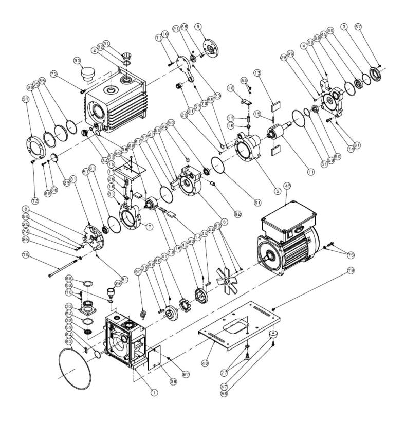
Fig. 12 Disassembly drawing of GLD-137CC oil sealed rotary vacuum pump
