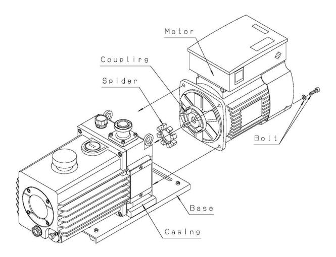
Fig. 11 Replacement of the coupling spider
