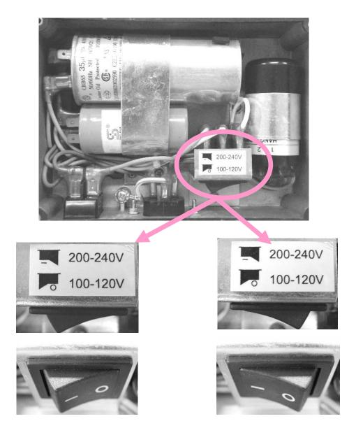
1-phase, 100-120V class power source 1-phase, 200-240V class power source Fig. 6 Changeover switch in the terminal box
