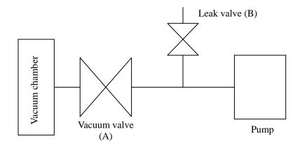
Fig. 5 Basic piping diagram to the vacuum chamber
