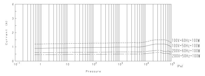
Figure 7. Characteristics of motor power
