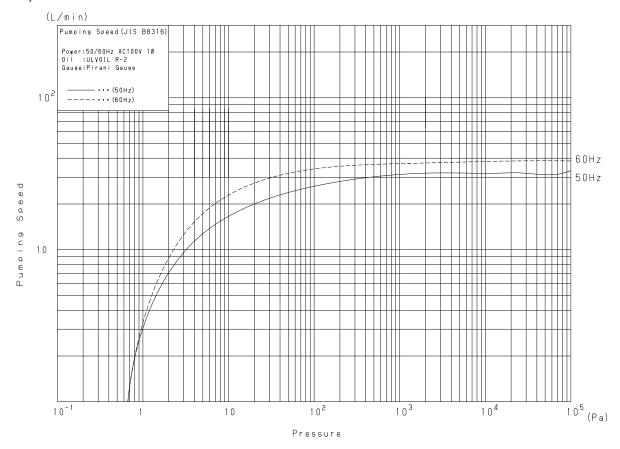
Figure 6. Pumping speed curve
