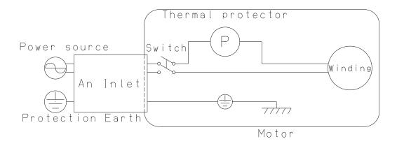
Figure 3. Electric wiring diagrams
