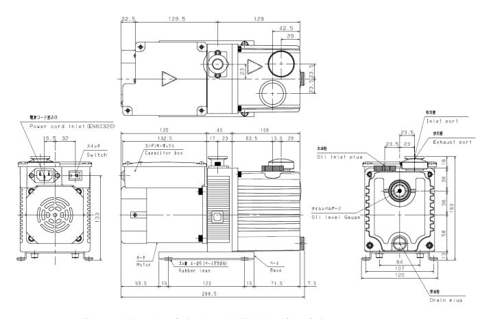
Figure 1. Dimensional drawing of GHD-031 oil sealed rotary vacuum pump.
