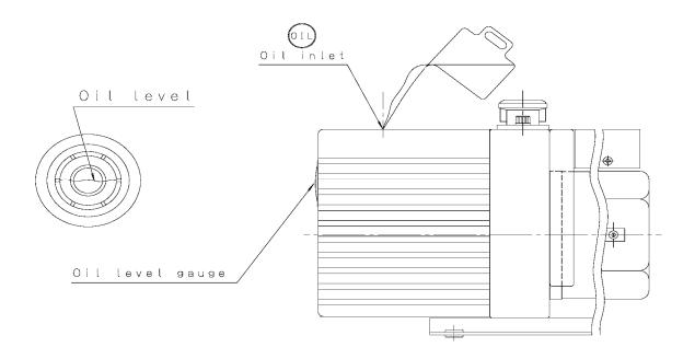
Figure 8. Lubrication of the oil sealed rotary vacuum pump
