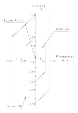
Figure 5. Change region of the voltage and frequency
