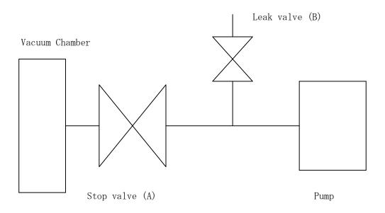
Figure 2. Basic piping diagram to the vacuum chamber
