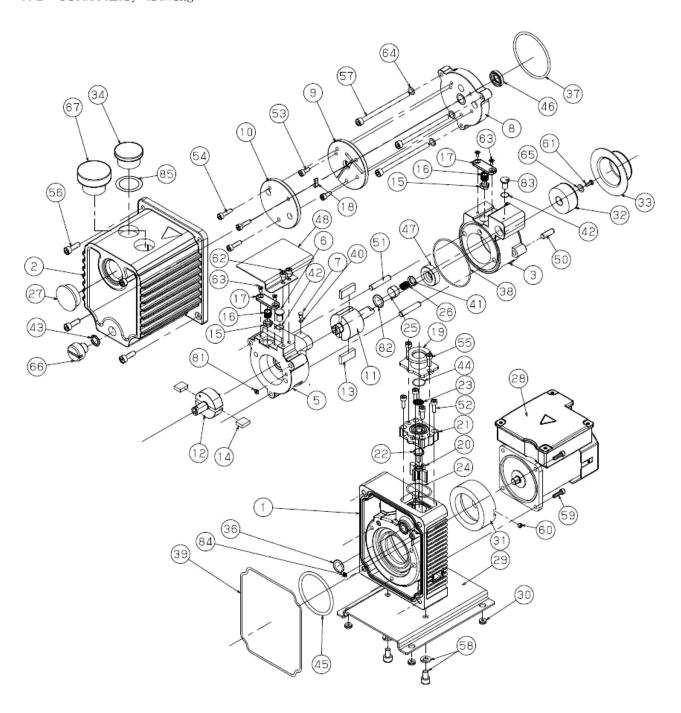
Figure 9. Disassembly drawing of GHD-031 oil sealed rotary vacuum pump
