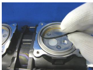
Photo 3: O-ring (S-67) removal
