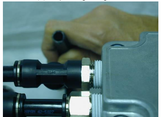
(10) Fitting the connecting tube.
