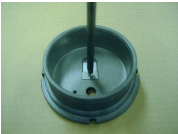
(4) Fitting the inlet valve
