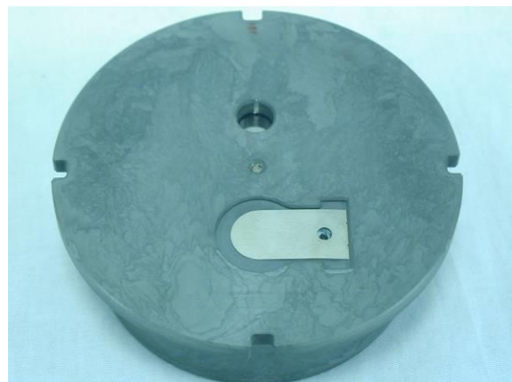
(4) Fitting the outlet valve
