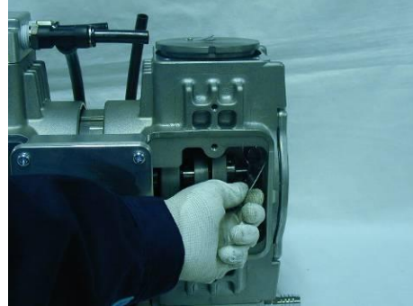
(2) Turn the fan upwards.
