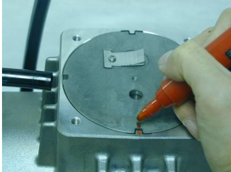
(1) Mark the casing and cylinder.
