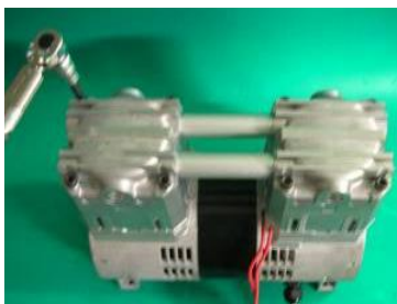
Photo 1: Pump-head disassembly, installation
