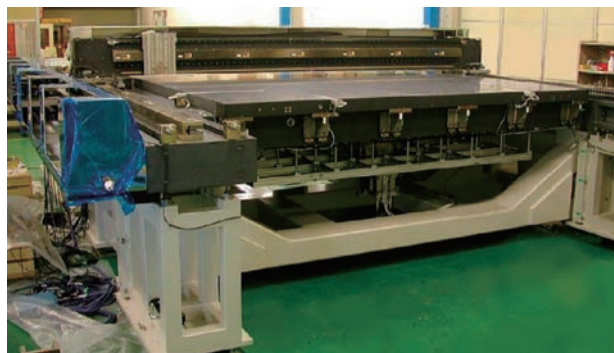
Figure 1-2 Appearance of a Gantry Type Stage
